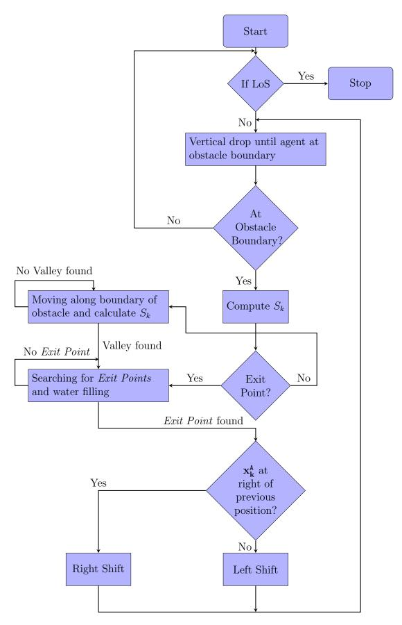
Figure 3.7: Flowchart of LoS by Water-Filling algorithm
