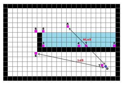
Figure 5.4: LoS by Water-Filling implemented in GMS
