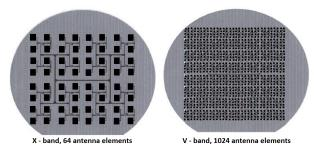
Figure: Wafer-scale antenna: 64 elements in 8-12GHz (left) and 1024 elements in 50-75GHz (right), Source: [Moh06]
