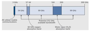
Figure: Millimeter-wave spectrum, Source: [ZK11]
