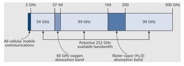
Figure: Millimeter-wave spectrum, Source: [ZK11]
