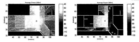
Figure: Variation in Received Power with 32mW transmit power at 5.1GHz (left) and 60GHz (right), Source: [WAN97]
