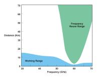
Figure: Working range and frequency reuse, Source: FCC OET Bulletin 70a
